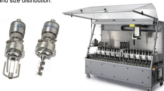
Figure 1: Chemspeed AutoPlant (left); reactors with anchor or triple helix stirrers (right).
